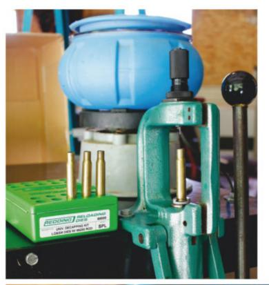
A Universal Decapping Die will remove spent primers from your cases before you resize them, allowing the primer pockets to be cleaned, keeping dirt and debris out of your resizing die.
