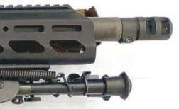
Carbon-fiber barrels can get quite thick without getting heavy. Note just how thick and stout the X-Caliber 6.5mm barrel is compared to the other two.
